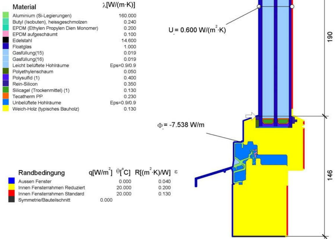
$$\psi = \frac{\Phi}{\Delta T} - U_g \cdot b_g - U_f \cdot b_f = \frac{7.538}{20.000} - 0.600 \cdot 0.190 - 1.492 \cdot 0.146 = 0.045 \text{ W/(m·K)}$$
