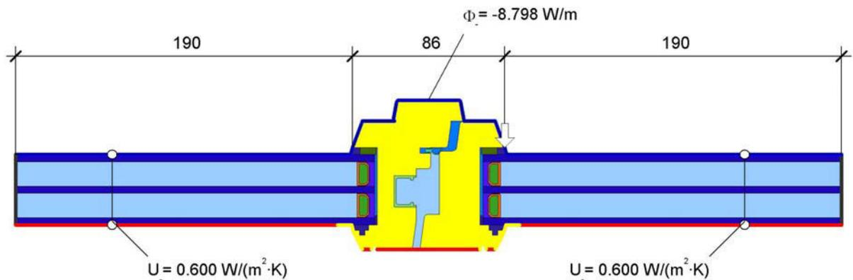
$$\psi_1 = \frac{\Phi}{\Delta T} = \frac{U_{g1} \cdot b_{g1} + U_f \cdot b_f + U_{g2} \cdot b_{g2}}{2} = \frac{8.798}{20.000} = \frac{0.600 \cdot 0.190 + 1.433 \cdot 0.086 + 0.600 \cdot 0.190}{2} = 0.044 \text{ W/(m} \cdot \text{K)}$$
