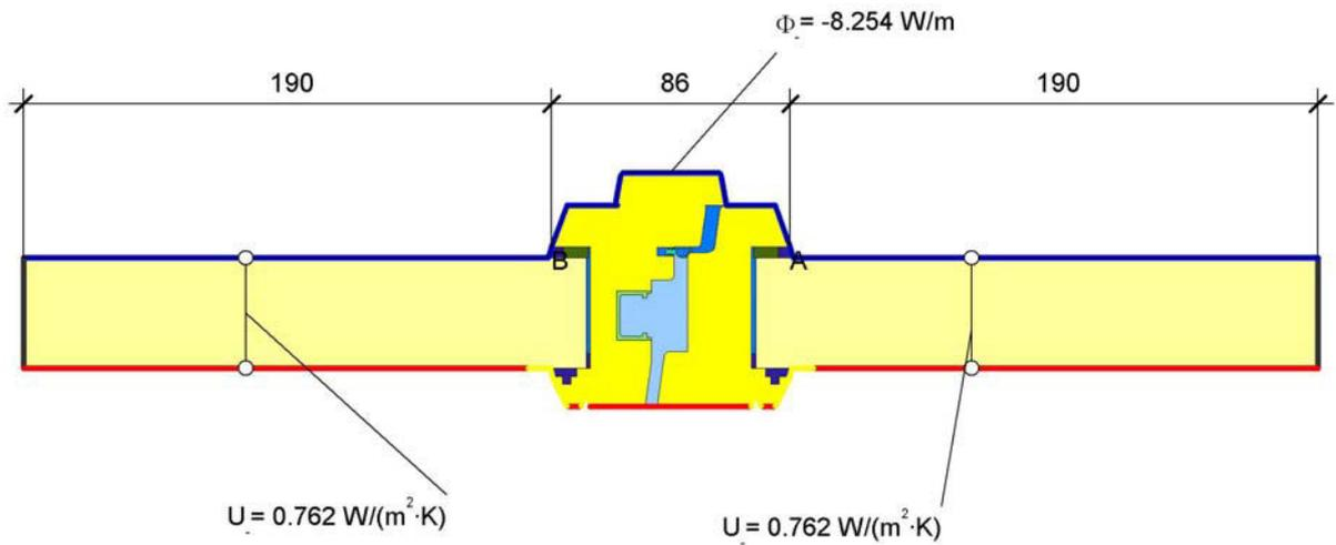
$$U_{fA,B} = \frac{\frac{\Phi}{\Delta T} - U_{p1} \cdot b_{p1} - U_{p2} \cdot b_{p2}}{b_f} = \frac{\frac{8.254}{20.000} - 0.762 \cdot 0.190 - 0.762 \cdot 0.190}{0.086} = 1.433 \text{ W/(m}^2 \cdot \text{K)}$$
