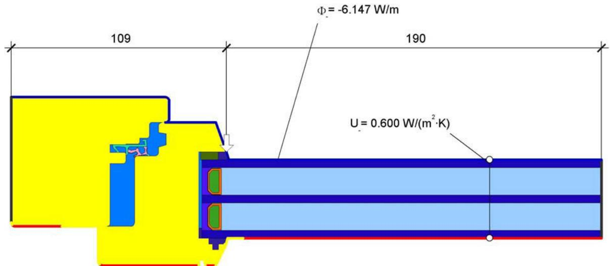
$$\psi = \frac{\Phi}{\Delta T} - U_g \cdot b_g - U_f \cdot b_f = \frac{6.147}{20.000} - 0.600 \cdot 0.190 - 1.352 \cdot 0.109 = 0.046 \text{ W/(m}\cdot\text{K)}$$
