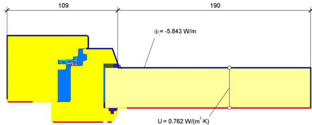
$$U_{FA} = \frac{\frac{\Phi}{\Delta T} - U_p \cdot b_p}{b_f} = \frac{\frac{5.843}{20.000} - 0.762 \cdot 0.190}{0.109} = 1.352 \text{ W}/(\text{m}^2 \cdot \text{K})$$
